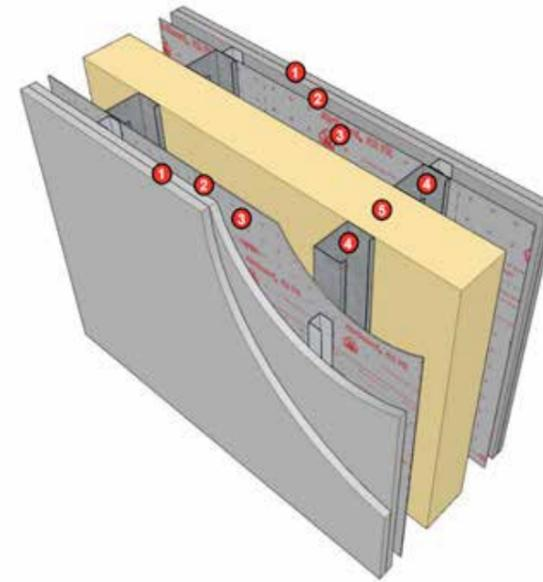
This diagram shows a Double-stud SFS separating wall, suitable for lightweight steel frame houses and apartments. A flexible semi-rigid insulation fitted in the cavity, separates the twin steel frames. Either side is AirGuard® A2 FR AVCL providing airtightness, vapour control and fire safety, helping to maintain the individual air quality and energy efficiency characteristics between zones.
