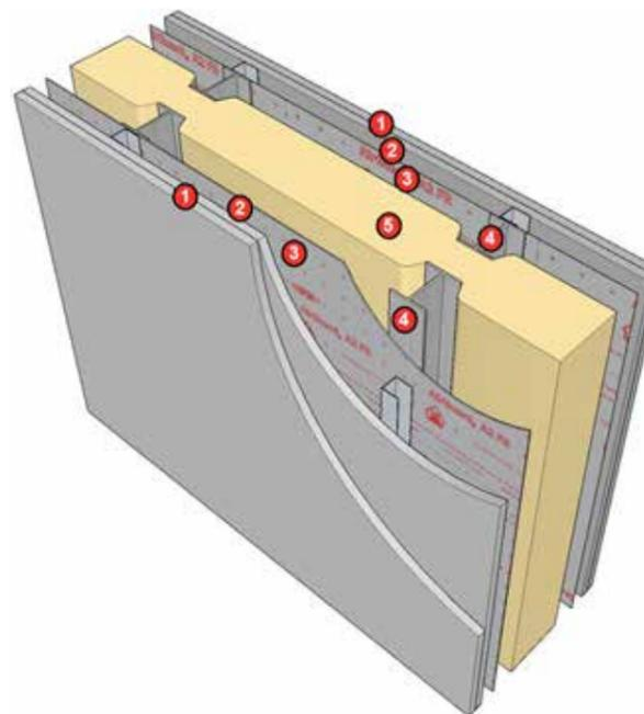
Diagram shows a steel frame 'Double-stud' separating wall system, which would **only be used with a reinforced concrete frame construction**. Components are similar to the previously shown lightweight system, but with a compressible semi-rigid insulation fitted in the cavity, separating the twin steel frames. AirGuard® A2 FR AVCL is installed on both sides to provide airtightness, vapour control and fire safety, helping to maintain the individual air-quality characteristics between zones.
