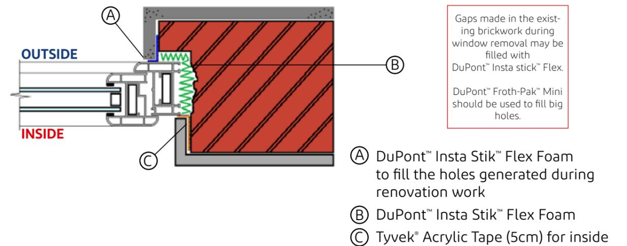
Gaps made in the existing brickwork during window removal may be filled with DuPont™ Insta stick™ Flex. DuPont™ Froth-Pak™ Mini should be used to fill big holes.
