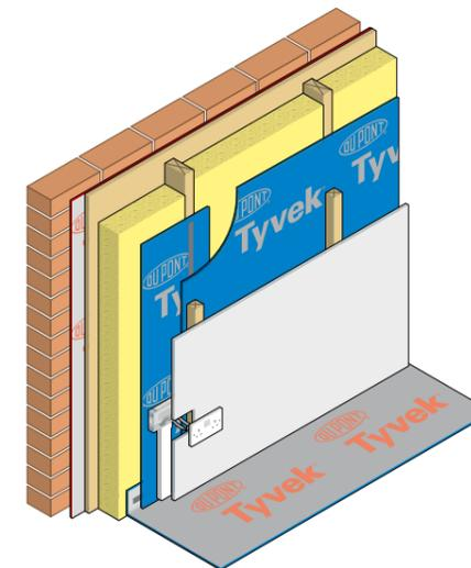
DuPont™ AirGuard® Control has been specifically developed for use as an air leakage barrier (ALB), but will also contribute in controlling the passage of vapour through a structure. Its use is particularly applicable in 'vapour open' wall constructions where external layers are of low vapour resistance.
