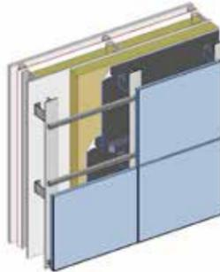
Vertical battens over the breather membrane have been included in some details to ensure positive drainage of moisture. Although they may not always be required they are recommended particularly in areas subject to extremes of weather.
