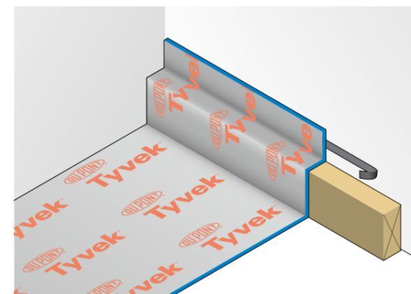
Fig. 36a - Wall junction - joists at right angles
