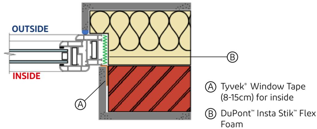
\* NOTE: Some external sealing provisions may not be necessary if the external insulation is being fitted immediately after the window unit.
