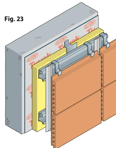
Where there is a risk of moisture penetration through the insulation and internal layers, a protection membrane behind the insulation is advised. The material to specify is dependant on the risk of condensation at this interface, determined in the main by the temperature. If in doubt a breather membrane should be used. In any case the material should be water resistant.
