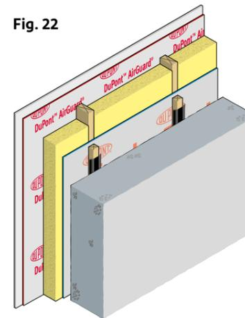
Battens should be fixed to the inside face of the existing wall via strips of DPC for protection against moisture. A new Tyvek® covered insulated panel can then be constructed away from the existing wall.
