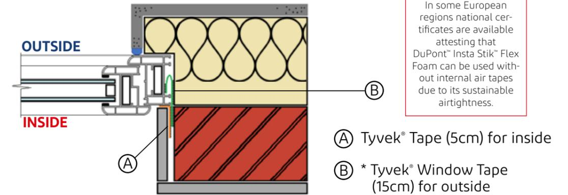
\* NOTE: Some external sealing provisions may not be necessary if the external insulation is being fitted immediately after the window unit.
