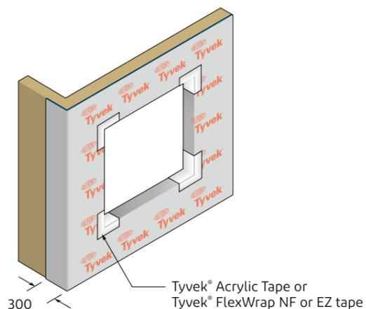
**Fig. 18 - Window head (render & lathe)**
