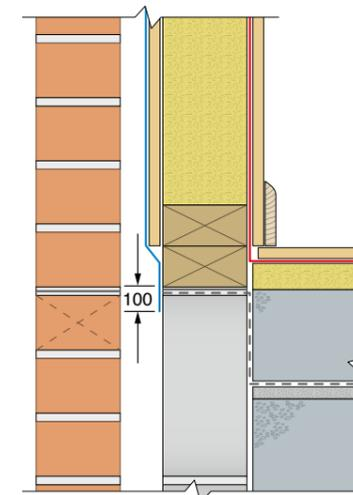
Application of the Tyvek® breather membrane follows the same process for each method and starts from the sole plate or bottom rail, working upwards.
