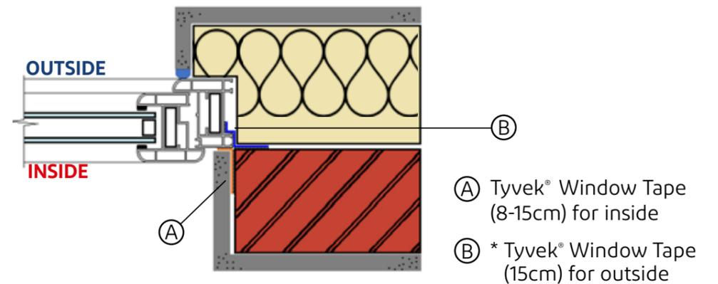
\* NOTE: Some external sealing provisions may not be necessary if the external insulation is being fitted immediately after the window unit.
