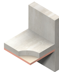
Insulation for structural ceilings (soffits)
