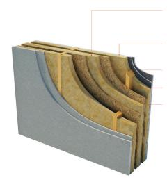
Wall width: 240mm (min) between inner faces of wall linings. 50mm (min) gap between studs (must not be bridged by any diagonal bracing).
