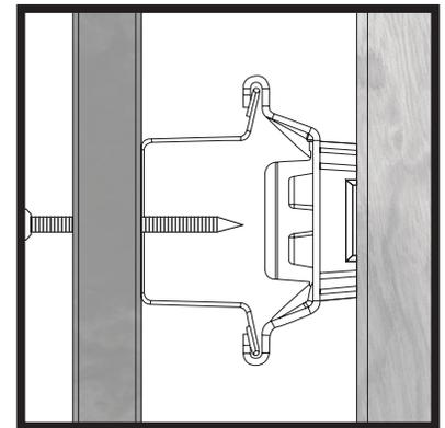
**NOTE** It is impossible to "short circuit" the **GenieClip RST** System when the correct screws are used. Should the installer hit a clip location, they will not be able to 'seat' the screw. They will be forced to move left or right on the track away from the **GenieClip RST**.
